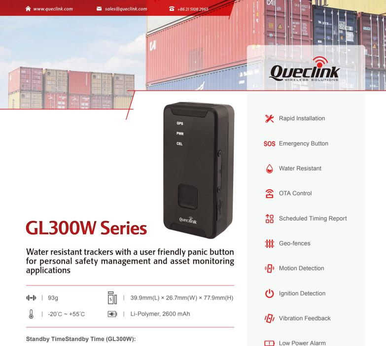
The GL300W series includes two GPS trackers that are designed for lone worker safety and asset monitoring applications. The ergonomically designed button makes the series ideal for applications requiring rapid emergency alert or instant geo-fencing based on current location. The series supports both 2G and 3G network for a wide application across the world.
